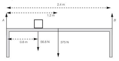
Select the left leg of the table A as the pivot. Sum of clockwise moments = sum of anticlockwise moments.  $(56.8 \times 0.8) + (375 \times 1.2) = (B \times 2.4)$  B = 206 NTotal weight = 56.8 + 375 = 431.8 N In equilibrium so A + B = 431.8 NA = 431.8 - 206 = 225.8 N
